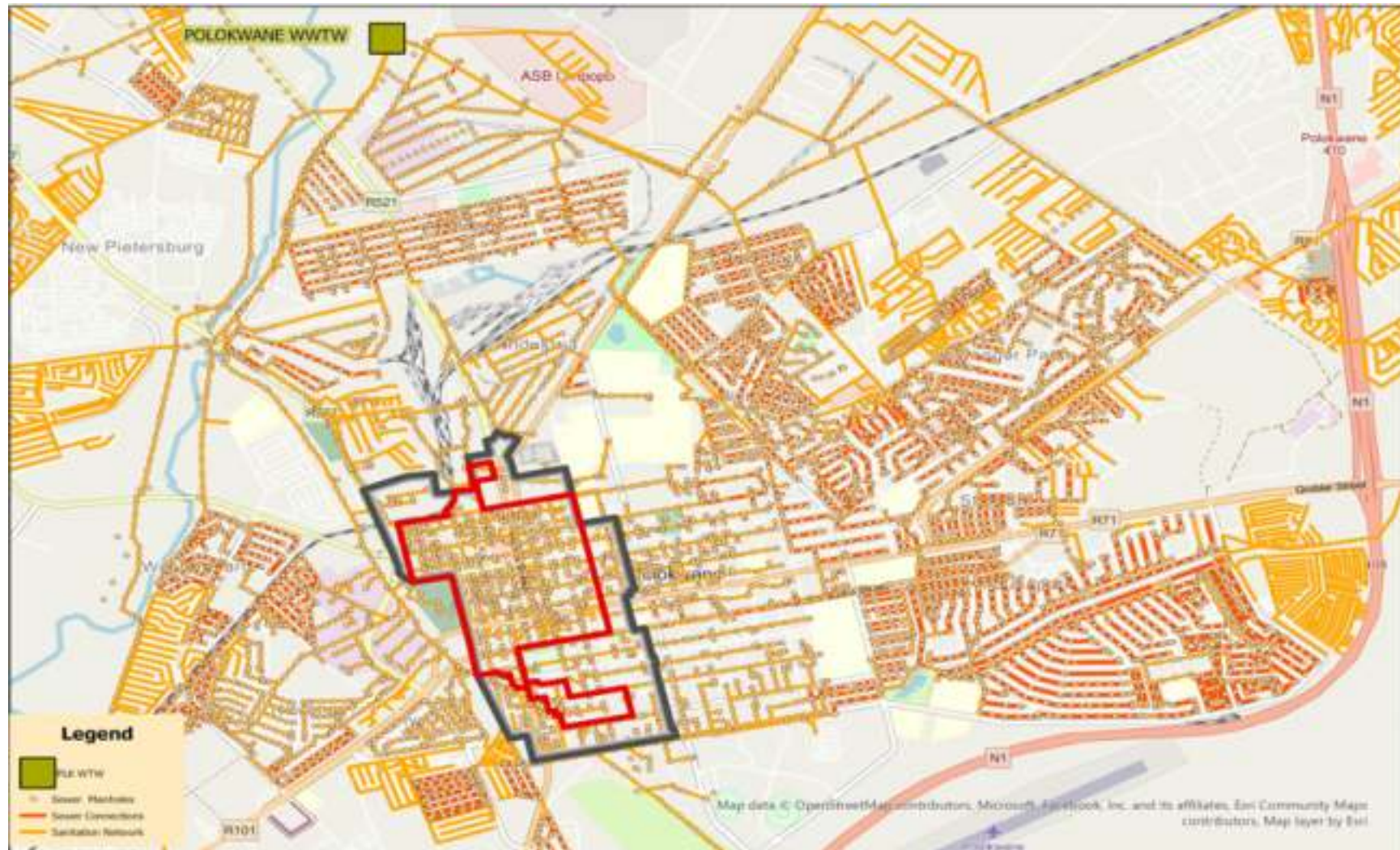
Diagram 173: Existing sewer reticulation network in the Polokwane CBD
