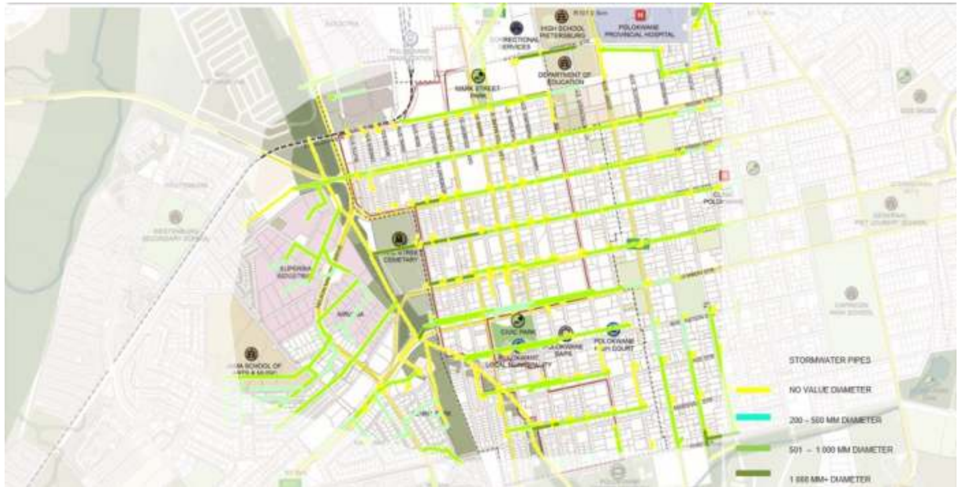
Diagram 175: Existing stormwater reticulation network in the Polokwane CBD
