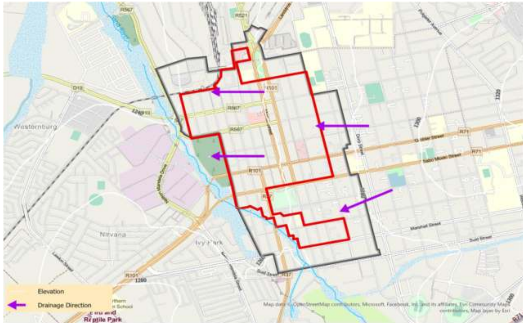
Diagram 174: Catchment Delineation & General Drainage Directions
